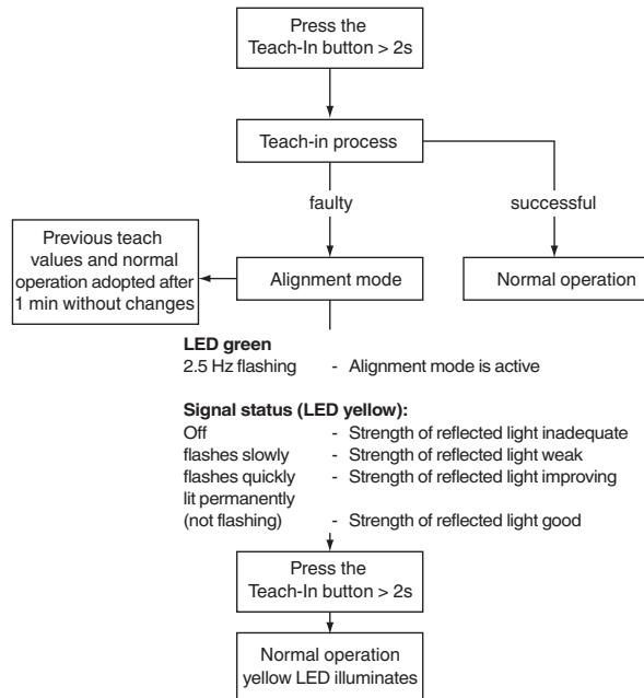
More stringent adjustment requirements: Ensure that the device is correctly aligned in the near range of 0.2 m ... 0.6 m.
